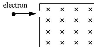
2. An electron enters a region that contains a magnetic field directed into the page as shown. The velocity vector of the electron makes an angle of  $30^\circ$  with the  $+y$  axis. What is the direction of the magnetic force on the electron when it enters the field?
